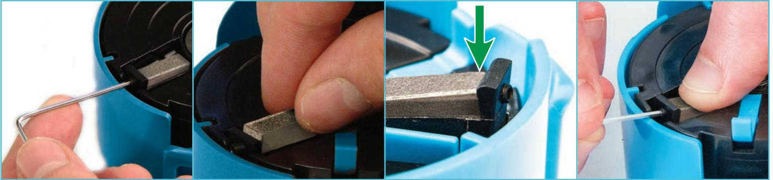
1. Slightly loosen the screw but **do not completely remove the screw.**
