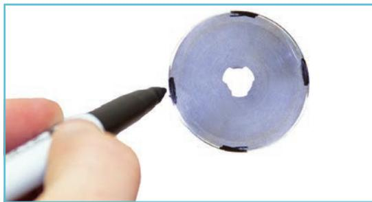
If your blade does not appear to be sharpening, mark the edges of the blade with a marker. If sharpening wears the marks away from the beveled edge, the sharpener is working.
