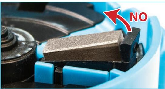
Make sure the stones are placed all the way down in their holders. If part of the stone is raised, or not all the way in, it will not sharpen your blade.
