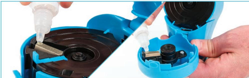
1. Make sure the sharpener is plugged in. Apply one drop of oil to both the top stone and the bottom stone. Add an additional drop of oil for every 60 seconds of sharpening.
