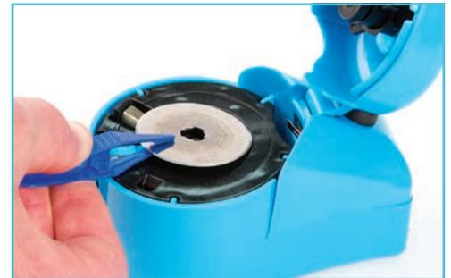
2. Using the blade handlers, place the blade in the blade tray. Make sure the blade is centered.
